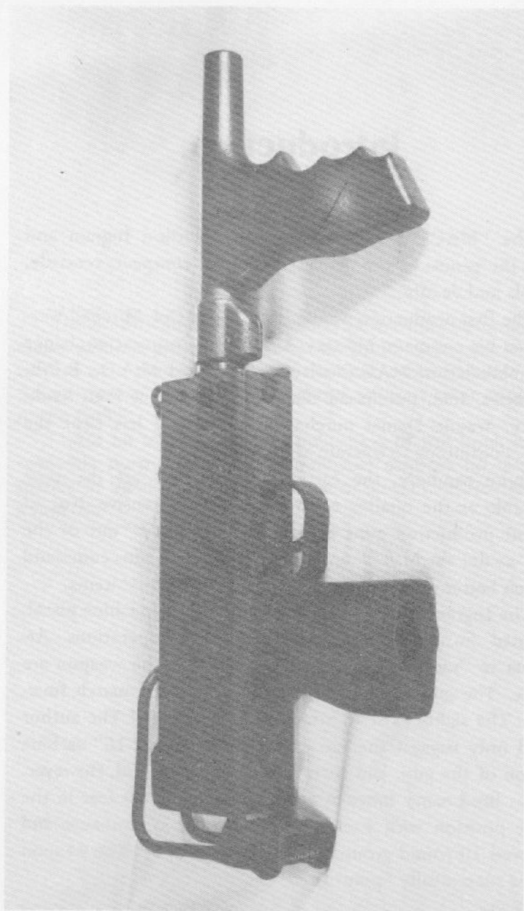
Pre-1972 MAC 10 from the author's collection. Note cast, position-adjustable hand grip.
