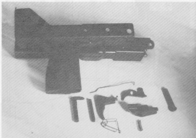
Detail stripped .45 ACP selective fire MAC 10 (less upper receiver). Note selector (far left, bottom row) which is, of course, non-existent in semi-auto model.
